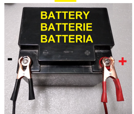
Find a battery of the type indicated below and connect it to the control unit with the supplied pliers: red (+) / black (-)
